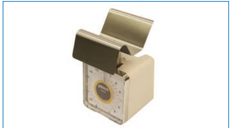
8417 Mechanical Portion Scale ..... $49 • Contoured stainless steel platform holds bagged items: fries, tacos, shrimp • Easy to read dial • 16oz. Capacity (Graduation 0.25 ounce) • Compact, space-saving design
